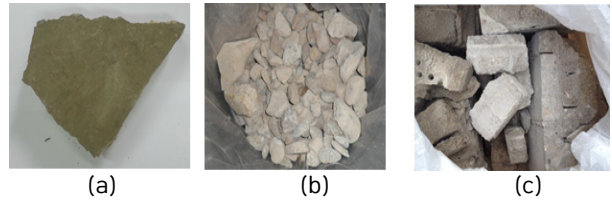
Fig. 1. Concrete wastes from (a) floor, (b) underfloor, and (c) wall.
