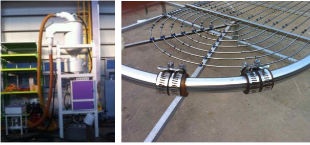
Fig. 2. High Pressure Blast Machine Unit. (Left) Fig. 3. U-Bend heat exchange tube Mockup. (Right)
