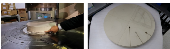
Fig. 4. Engineering-scale bentonite block (D760mm) manufactured from press and CIP.
