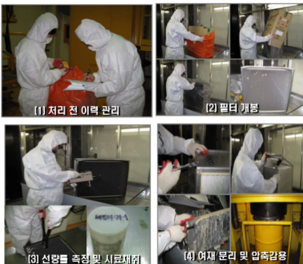
Fig. 2. Treatment procedure for spent filter at KAERI.
