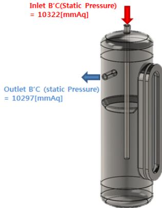
Fig. 2. Boundary Conditions for Seal Pot.
