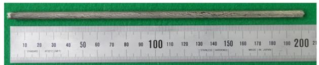
Fig. 1. Volatile U-10wt%Zr-5wt%Mn fuel slug fabricated by modified injection casting.
