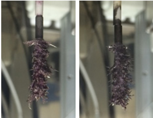
Fig. 2. Electrodeposited Uranium on Mo(left) and W(right) cathodes in 500^\circ\text{C} LiCl-KCl-3wt% \text{UCl}_3 molten salts. A constant current of -200 \text{ mA} was applied.
