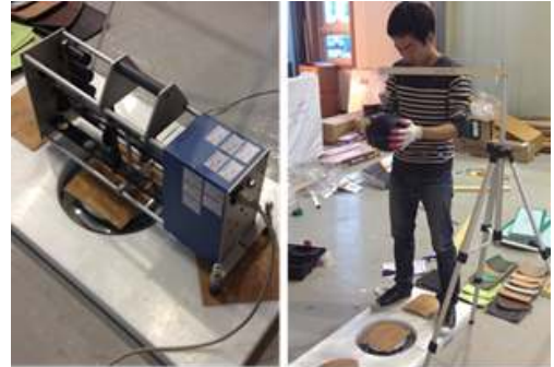
Fig.2 Measurement of impact force for floor finishing materials
