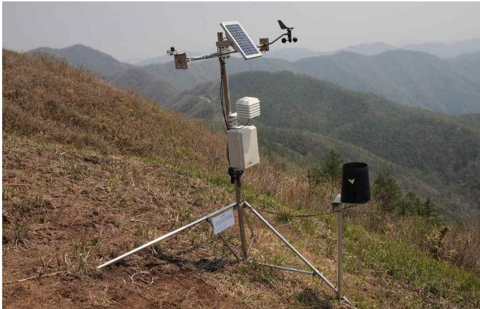
Fig. 5. An automated weather station installed at a mountain top location in the study area. It collects air temperature, humidity, wind speed, wind direction, rainfall amount and solar radiation at 1 minute interval and transmits the data to the laboratory via cell phone service every 10 minutes.
