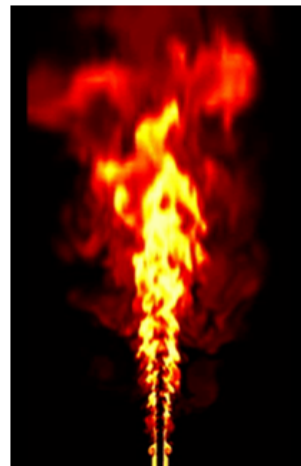
Fig. 3 Temperature contour of piloted CH 4 -air flame
