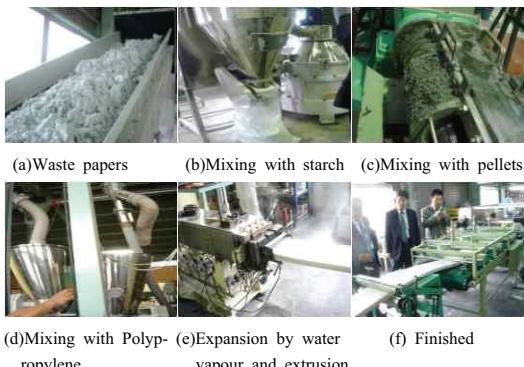
**Fig 1. Manufacturing process of the absorber**
