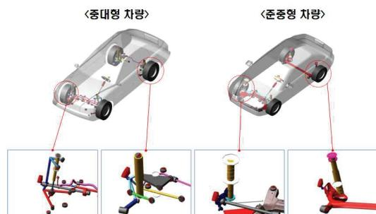
Figure 1. Multi-body vehicle dynamic model
