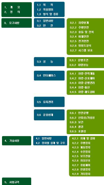
Fig. 5 Construction(draft) of technical specifications of railway vehicles
