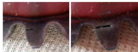
(a) Crack 2mm (b) Crack 4mm
