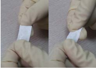
Fig 2 Fabricated BaTiO 3 -PEBA composite
