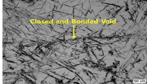
FIGURE.4 The microstructure obtained after 2 st incremental upsetting
