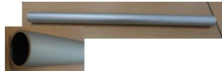
Fig. 6 Extruded hollow tube(non-homogenized billet)
