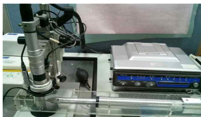
Fig. 1 A photo of the compact material testing machine developed for this study along with an electronic microscope
