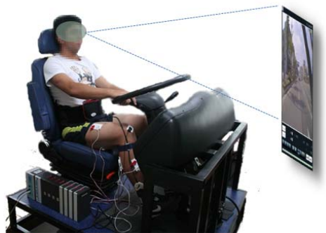
Fig. 1 Virtual driving system
