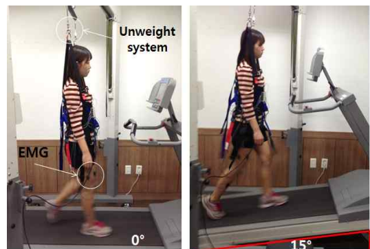
Fig. 1 Gait training with slope as 0° and 15° according to unweight protocol as 0%, 20% and 40%
