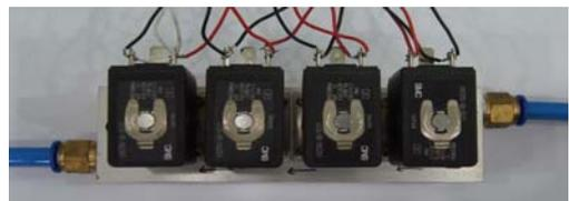
Fig. 1 Solenoid valve for fall guidance
