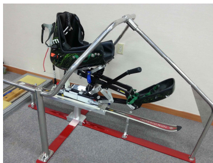
Fig. 1 The actual figure of the chair monoski simulator which developed from KOREC
