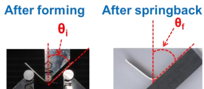
Fig. 2 Angles after forming and springback
