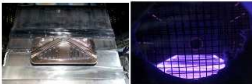
Fig. 3 Fabrication of die surface coating by DLC
