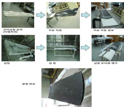
Fig. 4 Manufac. process of Coreless Core
