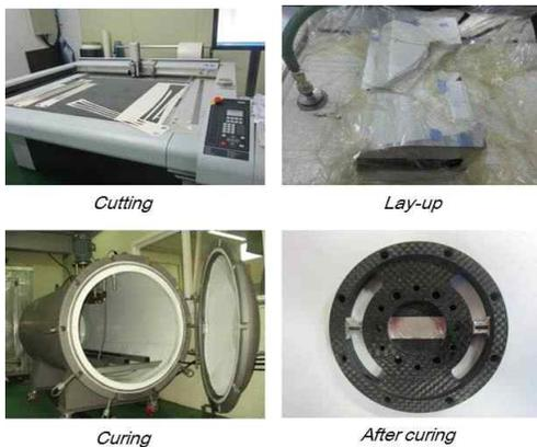
Fig. 2 Curing cycle and manufacturing procedures
