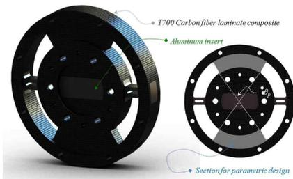
Fig. 3 Design parameter of transducer frame
