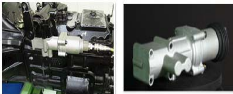
Fig. 2 Transmission(left), Power Shift
