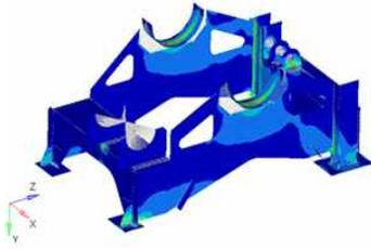
Fig. 3 The FEA result of the topology optimization modify model
