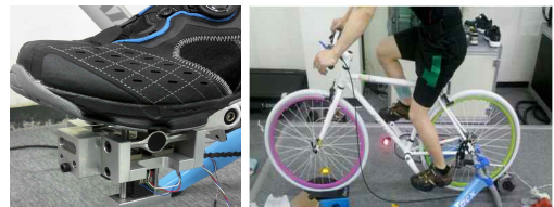
Fig. 1 Measurement of pedaling load on riding
