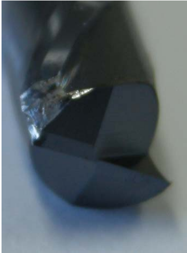
Fig. 3 Broken milling cutter after milling
