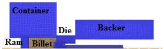
Fig. 2 FE analysis model and porthole die
