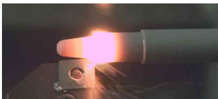
Fig. 1 Machining from the turning of laser preheated silicon nitride
