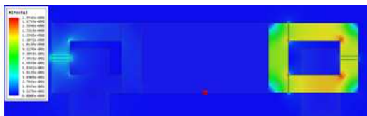
Fig. 4 Magnetic flux density analysis of radial HMB with 10A current
