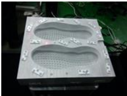
Fig. 2 Shoe mold for 3-D scanning
