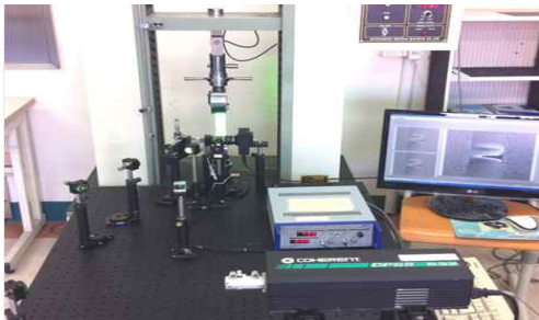
Fig. 3 Photography of Shearography setting
