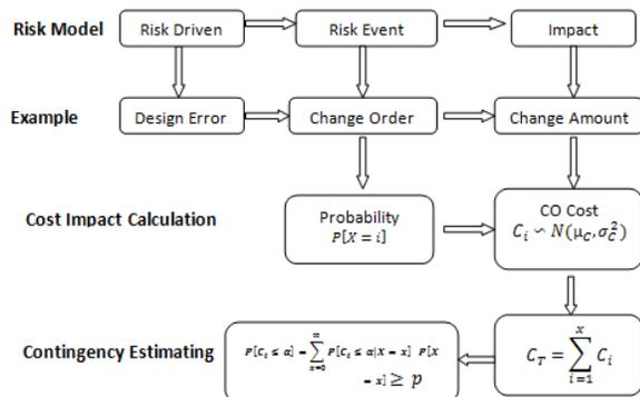
Figure 3 Probabilistic Contingency Calculation Model
