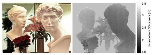
Figure 3. Captured 14Mp color (left) and full HD and depth (right) images
