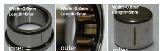
Figure 7. Kind of the defected bearing
