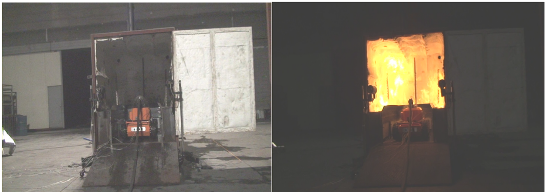
Figure. Test for Fire Protection of Fire Fighting Robots
