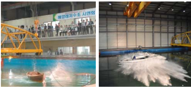
Fig. 1 Photograph of Pleasure Boat's Drop Test
