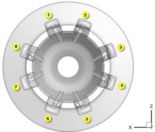
Fig. 4 Rear View of Solid Rokcet Motor with Secondary Injection Valves and Pipes. Attached Numbers are Each Valve Number.
