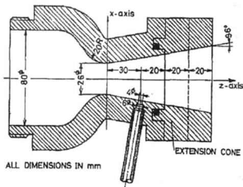
Fig. 1 Schematic of supersonic cone type nozzle with secondary injection orifice[4]
