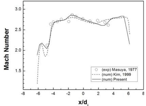
Fig. 2 Mach number along x-axis at  $z=70\text{mm}$
