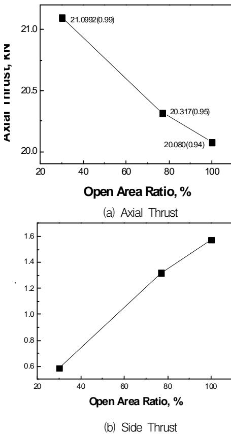
Fig. 5 Axial Thrust and Side Thrust along Valve Open Area Ratio.
