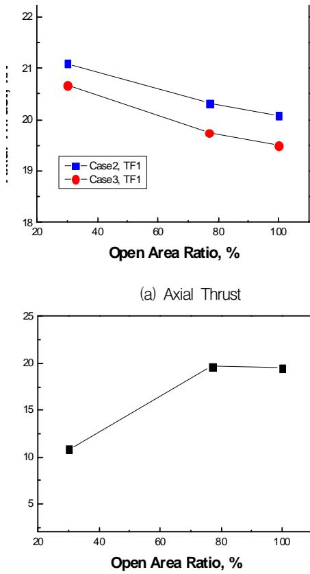
Fig. 6. Axial Thrust and Roll(Y-axis) Moment along Valve Open Area Ratio.
