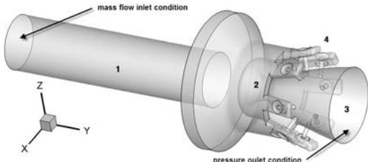
Fig. 3 Schematic of Solid Rokcet Motor with Secondary Injection Valves and Pipes
