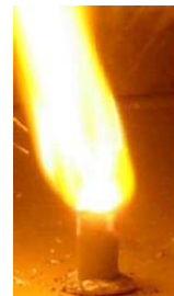
Fig. 4 Combustion of aluminum sample in the soft shell with water.
