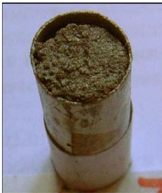
Fig. 2 Sample of 12mm diameter with composition Al/H 2 O=1:1
