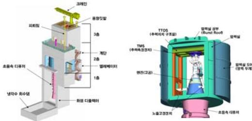
Fig. 7 3D Modelling of Test Stand for High Altitude Rocket Engine Test Facility(HARETF)
