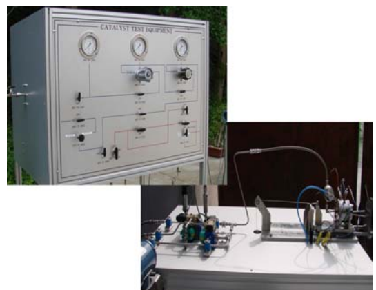
Fig. 2 Propellant supply & Thrust measurement system
