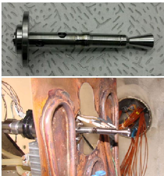
Fig. 2 1N Thruster Development Model and Firing Test
