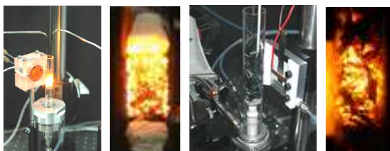
Fig. 3 Combustion in porous SiC media of foam(a), wrapped felt(b) and chopped fiber(c,d)
