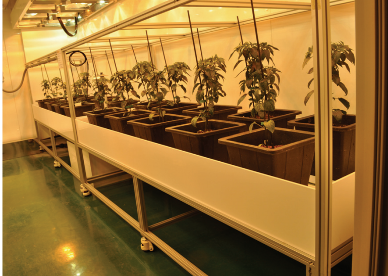
Fig. 5. Subirrigation system in the walk-in growth chamber
