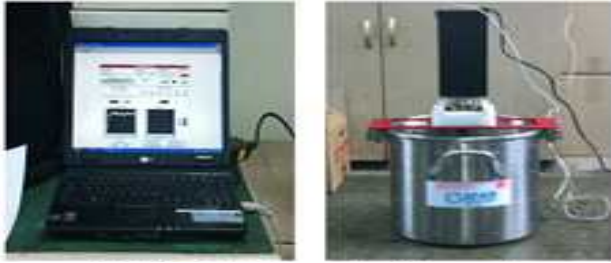
Figure 1. Rheology test for concrete
