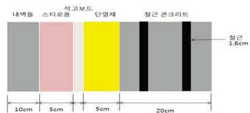
Fig. 1. Section of apartment structure.
